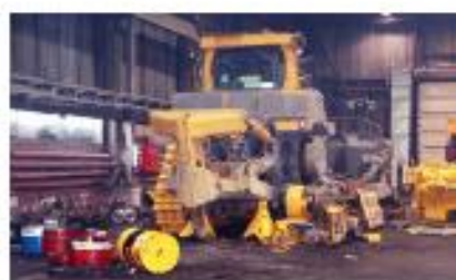
HS30035 jack stand supporting CAT bulldozer
