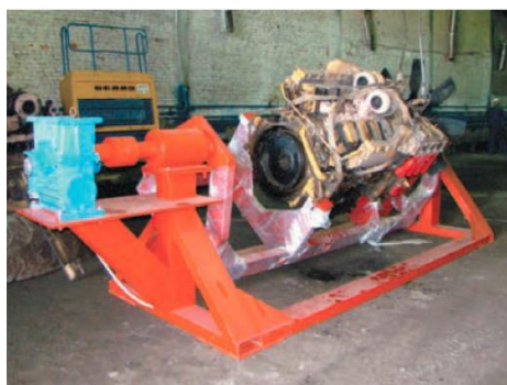
Rotating stand designed for assembly/disassembly of SAA12V140 engine on Komatsu HD785-5 dump-truck
