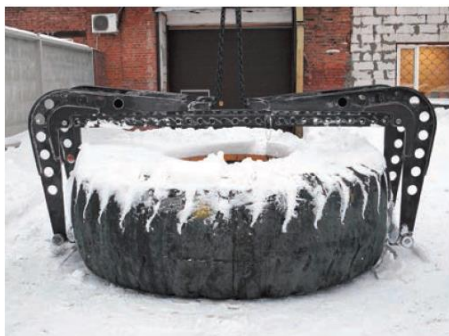
OTR wheel gripped by an «MKG» tool
