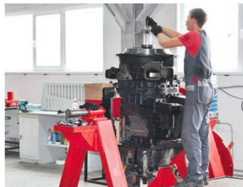
ALISSON TSA-100AE transmission assembly/disassembly rotating stand at work
