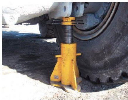
CM-M-series adjustable mechanical jack stand at work
