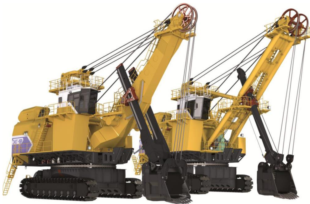
IZ-KARTEX Mining Shovels for working in complex with dump trucks of 75 – 360 t carrying capacity
