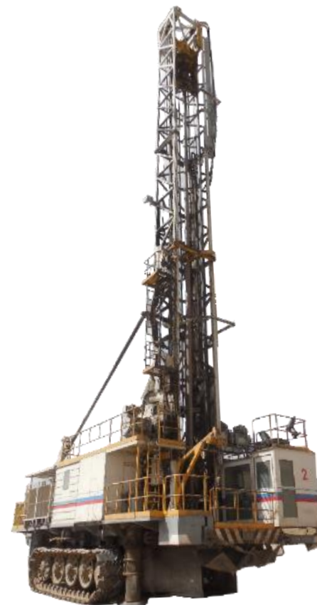
ROTARY DRILLING RIG SBSH -270AM WITH CRAWLER OF MULTI-SUPPORT TYPE
